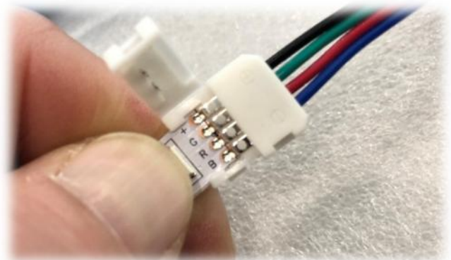
Figure 4. Gently Inserting the LED Strip into the Solderless RJ45 Adapter
