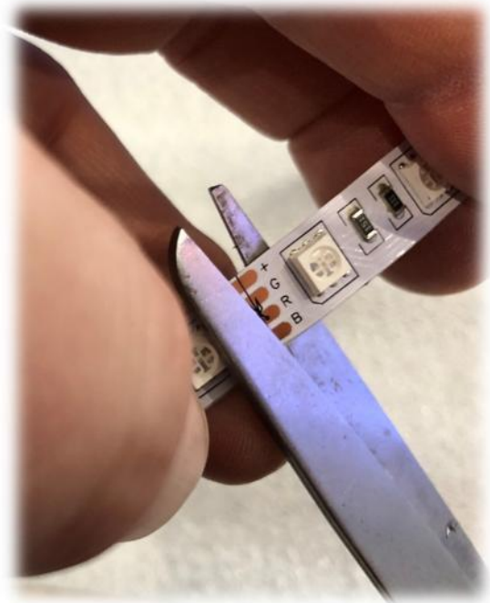
Figure 2. Cutting the LED Strip on a Designated Cut Line
