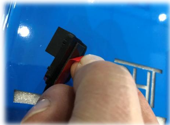
Figure 11. Peel The Backing From The Adhesive On The RJ45 Adapter And Stick In Desired Location.
