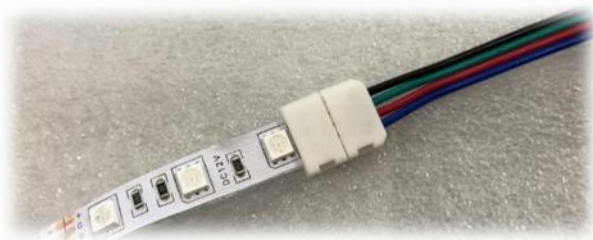
Figure 5. Lid Snapped Shut and LED Strip Held Firmly in Place by Connector
