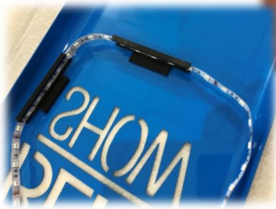
Figure 12. Finished Mounting LED Strip.
