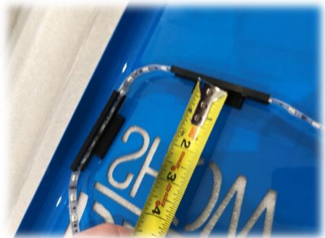
Figure 10. For Mounting To Illuminate An Opening, Keep The Strip About 2 Inches Away Where Possible So The Actual Strip Is Not Visible.
