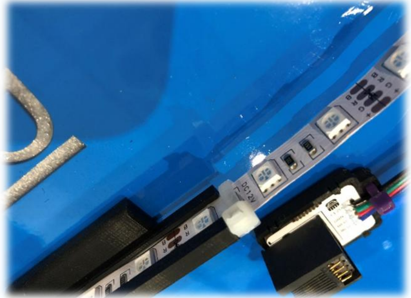
Figure 15. Zipties Can Also Be Used To Secure Any Loose Ends. It Is Important Not To Allow Any Of The Electrical Connections Short To Any Metal Surface.
