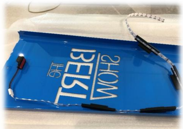
Figure 9. Laying Out the Strip with the Supplied Mounting Clips.
