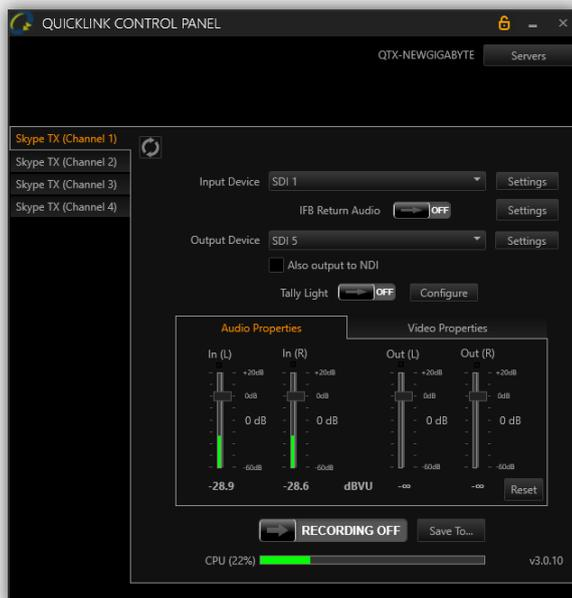
The Quicklink Control Panel will provide complete management and control of input and output settings for each individual caller.
