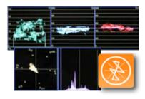
New tools have been included to assist in the signal monitoring, such as independent waveforms for Y, Cb and Cr, and vectorscope, displayed in different colours for a quick identification of each
