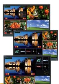
In addition to the standard quadsplit mode with four identical windows, there are different layouts available with several combinations of sizes and positions, along with the WFM tools.
