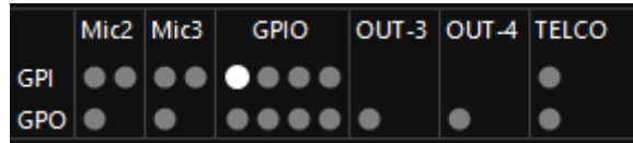
OXYGEN REMOTER displaying of the activated GPI 2
