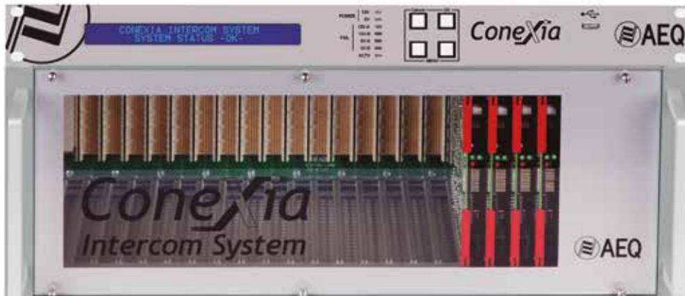
Conexia system structure is based on a 4U 19" rack that comprises three important blocks; at the front, the slots for the audio processing and communications crosspoints DSP cards are located. These tasks are performed dynamically, so backup cards for automatic function failover can be inserted.
