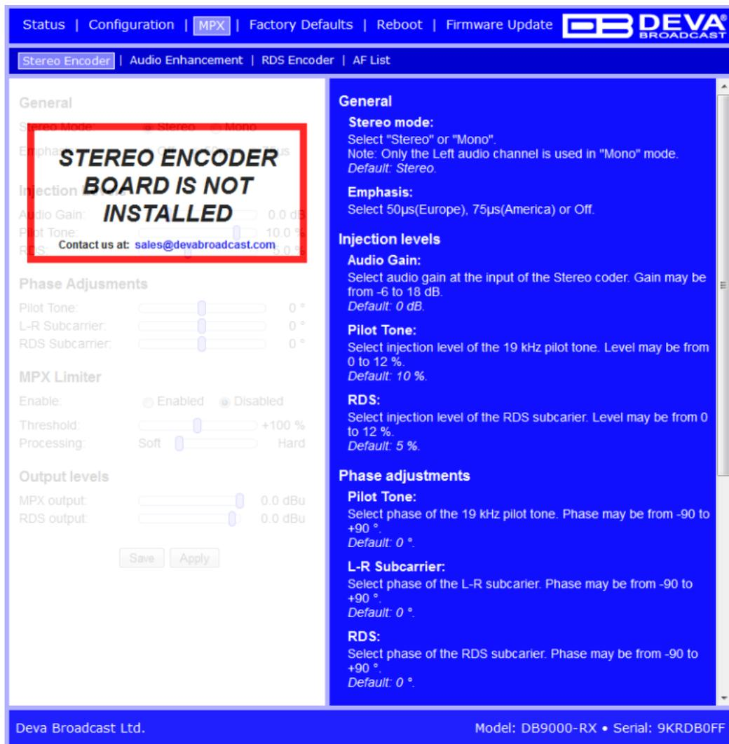
In this case, following strictly the previously described procedure, remove the equipment's lid (Steps 1 & Step 2) and make sure that the MPX board has been properly installed.
