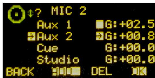
In the example, the send from "MIC 2" input to the summing bus "Aux 1" is linked to the fader (there is no arrow in the cross point) and the send to "Aux 2" is pre-fader (there is an arrow in the cross point).
