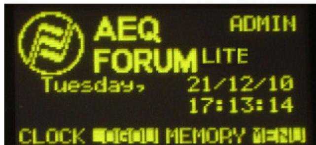
The four options visible on the last line of the display are associated with the four contextual keys below, from left to right:
