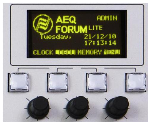
Among the general functions are the instant activation and adjustment of audio effects (EQ, filters, limiters, etc.), configurations and memories management, disconnection of applied effects, phase change, inserting of a test signal, as well as clock, timer and stopwatch for timing control, etc. For more information see chapter "3. DESCRIPTION OF THE INTERNAL MENU" of this manual.
