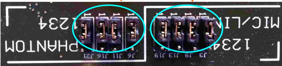
**IMPORTANT NOTE 1:** For each input, all jumpers associated with each option (mic/line or Phantom power) must be configured in the same position in both zones for a correct operation of the console. On the other hand, it's **VERY IMPORTANT** that the Phantom power activation is made (when needed) only in that/those input/s that are previously configured for microphone level.
