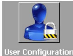
"User Configuration" submenu allows you to set access levels and create users to operate the AEQ FORUM LITE mixing Console.
