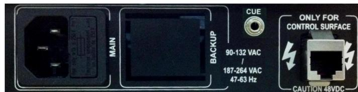
The console/engine data and power supply interconnection is located at the right of the power supply inputs. It is designed for use with straight Ethernet cabling, but also carries proprietary **power supply lines**. Please use the cable provided with the unit only. If necessary, this connection could be made by means of a cable of up to 250 meters, using a continuous CAT5E shielded (FTP) cable (or better) and checking that the shield is connected to the connectors case.
