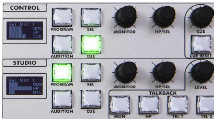
There are two distinct parts in this submenu: the upper part is dedicated to the configuration of the Studio Room section and the lower to the Control Room section.
