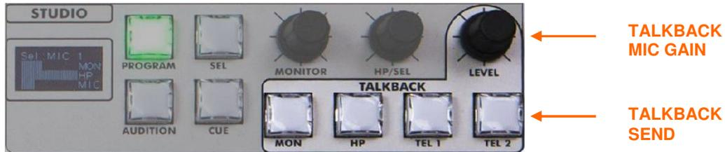
The talk-back section of the control surface consists of these 4 key buttons, working along with the volume adjusted by means of the "LEVEL" (Talkback Level) encoder.
