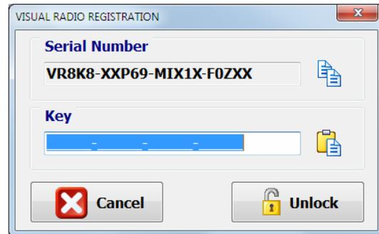
In case your order includes any of those functionalities, the console is supplied from Factory with the functionality activated. If you want to activate it a posteriori, you must copy the "Serial Number" by means of the associated button and send it to AEQ in order to generate the associated "Key" and send it back to you (you must paste it by means of the associated button).
