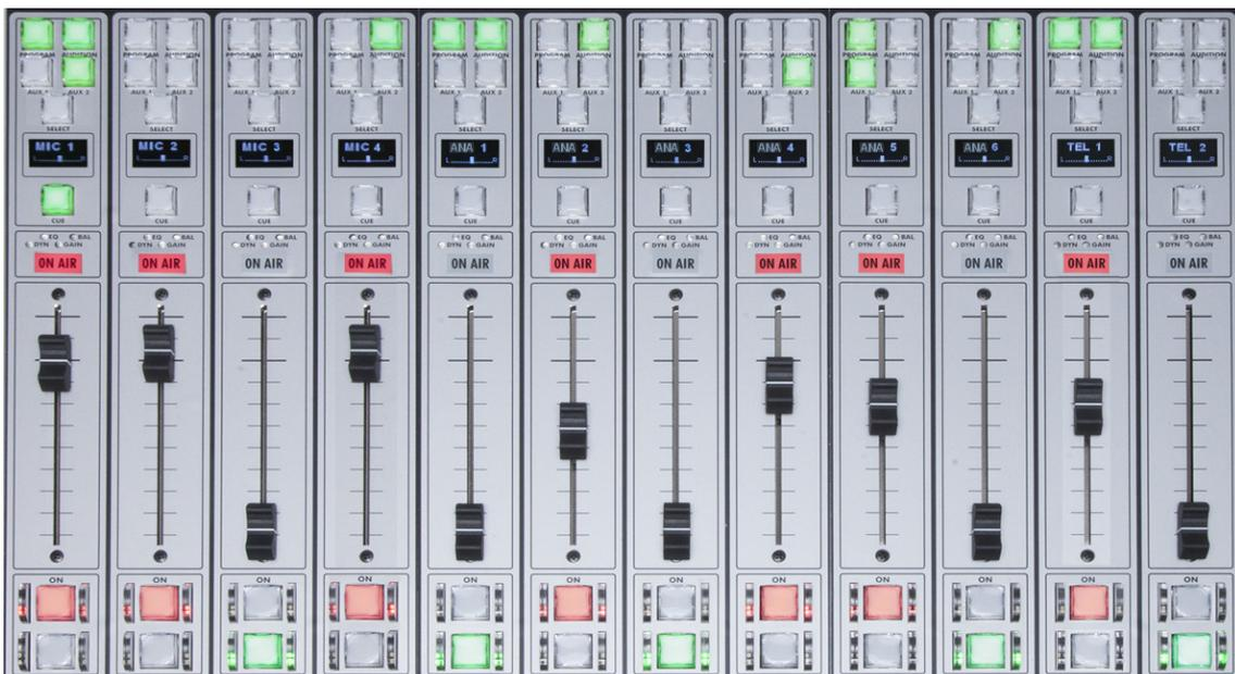
In this case, the "ANA 1" signal defines an operative **priority 1** because the "PROGRAM" routing key is activated (it doesn't matter that the "AUDITION" key is also activated and the channel is not active). "ANA 1", "ANA 2" and "TEL 2" signals will not be sent to "MPX 2" bus because they are excluded from the group.
