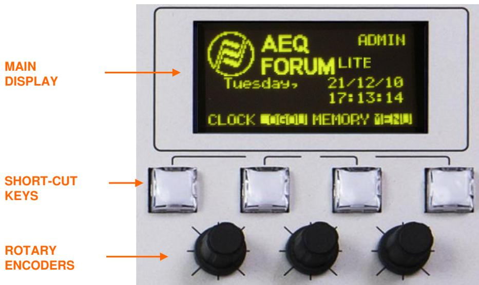
The three rotary encoders are related to the remaining lines of the menu. Each display is described in chapter 3 of this manual but the thumb-rule for the association of the rotary encoder to the visible functions is: option visible to the left or in the upper part of the menu is controlled from the encoder located to the left. In many cases the encoders are represented and labelled on the display for easy operation.
