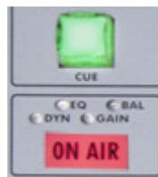
These four processes (EQ, dynamics, balance and gain) are controlled from the internal menu associated with the "SELECT" button on the main screen of the Control and Monitoring section.
