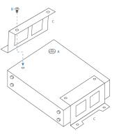
Use the four provided No. 6 screws ("D") and the four cup washers ("E") as shown in the diagram to the left to secure the Gadget to the plywood underside of the counter, desk, or table.
