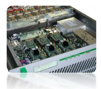
The optional digital processor can also provide re-multiplexing functions (with PID filtering, insertion / change of tables, etc.) and "seamless" switching between two transport stream inputs; in this way, when operating in SFN mode, the transmitter doesn't interrupt the emission when switches between input transport streams (from primary to secondary or vice versa).
