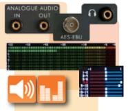
Audio monitoring is possible thanks to the different input options (analogue and SDI-embedded) and outputs (analogue, digital AES-EBU, headphones and stereo built-in speakers).
