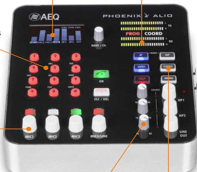
Listen level control for headphones 1/2 and line output with TX / RXbalance adjustment.
